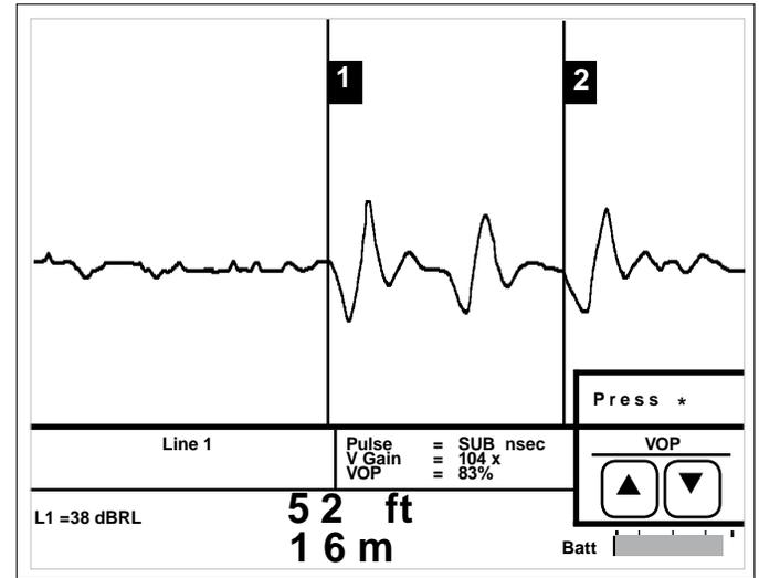
The horizontal zoom and vertical gain keys allow the operator to view these three crimps more closely.
