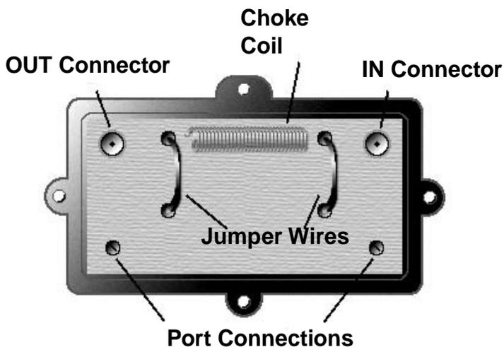
instead of the original tap plate to gain quick and easy access to the cable.
